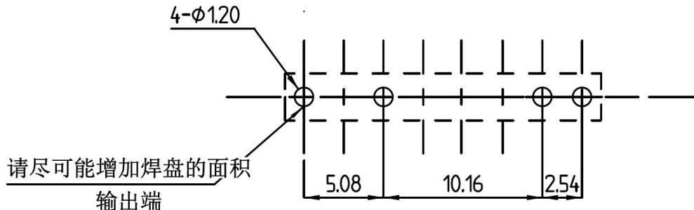
Please enlarge the solder pads of output. 推荐使用散热器 Heatsink is recommended
